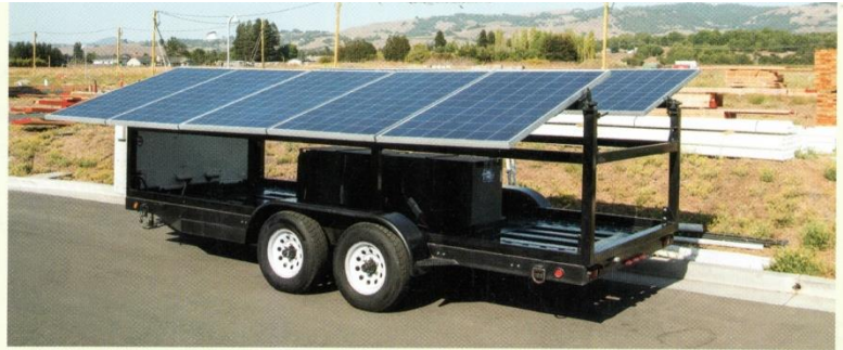
Watt Wagon solar power trailer (Lisa Rose Photography)
